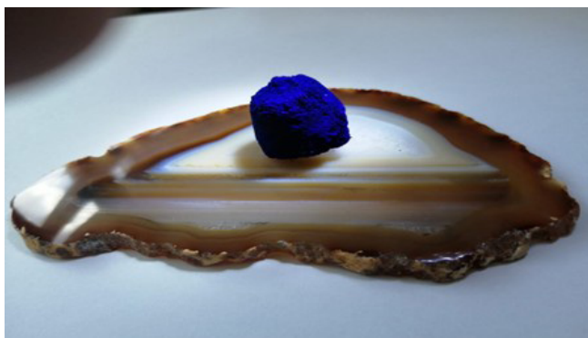
Figure 2 – A sample of blue ultramarine synthesized on the basis of the developed charge (Table 2) on a polished plate of agate.
